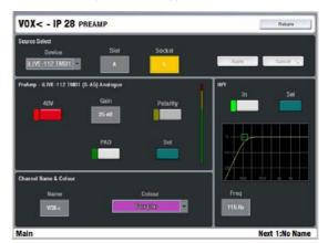
**Input patch bay** Select the input source for the channel from the Device drop down menu and press Apply to confirm. This lets you rearrange your patch according to how things are plugged up on stage, split signals into two or more channels, select from remote sources such as an EtherSound or ACE mic splitter and more. Channel sources include:
